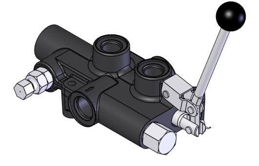
Model P81 Single spool Mono-block 80 l/min The P81 is an on/off directional control mono-block valve and is designed as a log splitter valve. It is directing the working fluid between hydraulic pumps and consumers (hydraulic cylinders, motors, etc.) and the tank. It has a spring centered in one direction, and pressure released detent in the other direction. Automatically kicks back to neutral when cylinder completes stroke. The P81 also includes built-in adjustable inlet relief valve.
